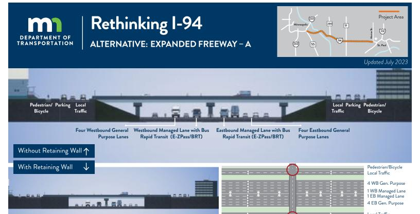
This concept involves rebuilding the existing freeway and adding 1 managed lane with bus rapid transit (BRT) in each direction. The BRT system could include up to three stops along the managed lane. The total number of lanes will vary because the current number of lanes also varies.
