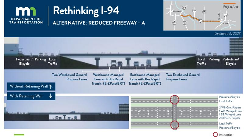
This concept involves rebuilding the existing freeway to include 2 general purpose lanes and 1 managed lane with bus rapid transit (BRT) in each direction. The BRT system could include up to three stops along the managed lane.
