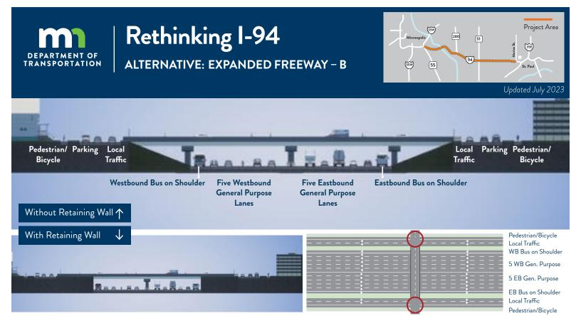
This concept involves rebuilding the existing freeway and adding 1 new lane (for all vehicles) and extending the bus shoulder along the entire corridor in each direction. The total number of lanes will increase.
